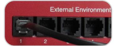
2. Connect the RJ-11 jack on the sensor cable to a digital sensor port on your Room Alert
